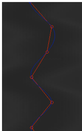
Figure 4.10: Plugin "Spline Tracking" - before (red) and after (blue) execution of the plugin
